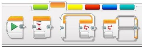
**Flow control tab:** Consider using a **wait for** or **switch** block to control the maximum and minimum tone range.
