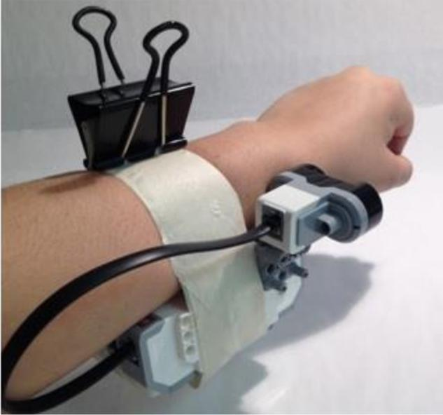
The above device uses an ultrasonic sensor. The user points it in a direction, and the device will beep if an object is close. This device will prevent the visually impaired user from bumping into objects.
