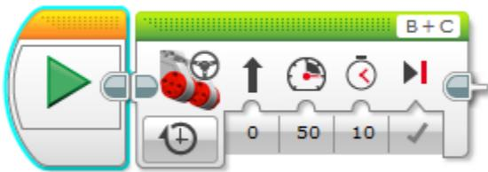
The above program moves two motors plugged into port B and C at 50 power for 10 seconds then brakes
